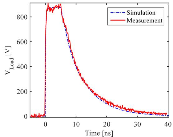
Fig. 2 Simulation and measurement of TLP voltage waveform.
