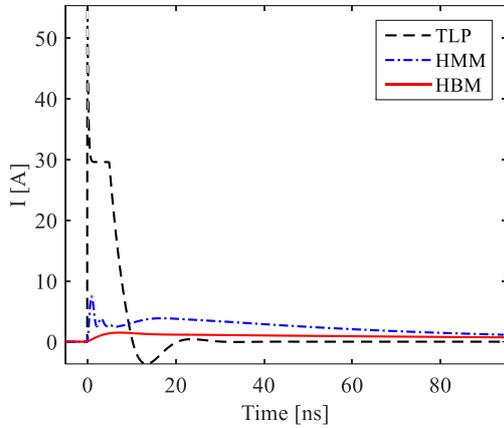
Fig. 3 Comparison between simulation of TLP, HMM, and HBM current waveform passing through 2  $\Omega$  load at 2 kV setting.
