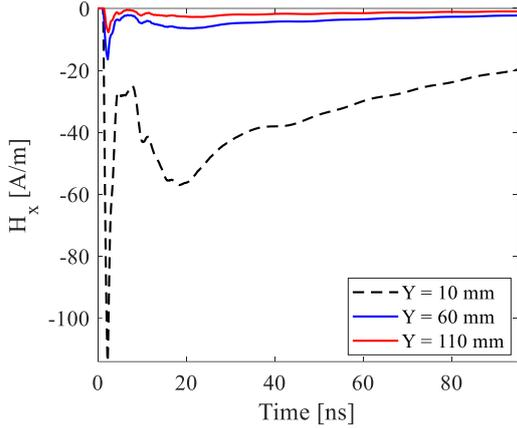
Fig. 6 Simulated magnetic field normal to microstrip line ( $H_x$ ) at different distances from ESD generator tip.
