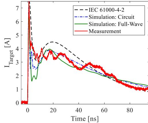
Fig. 1 Simulation and measurement of ESD generator current waveform.
