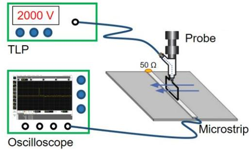
Fig. 5 Measurement setup for near-field injection using TLP.
