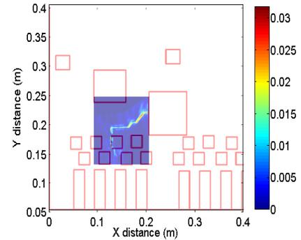
Fig. 5. Measured total tangential field component magnitude in dBm.
