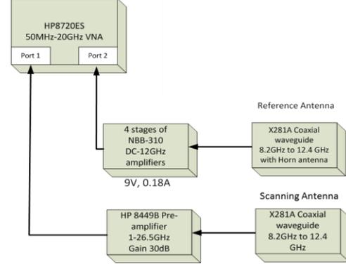
Fig. 3. The schematic diagram of the ESM measurement setup
