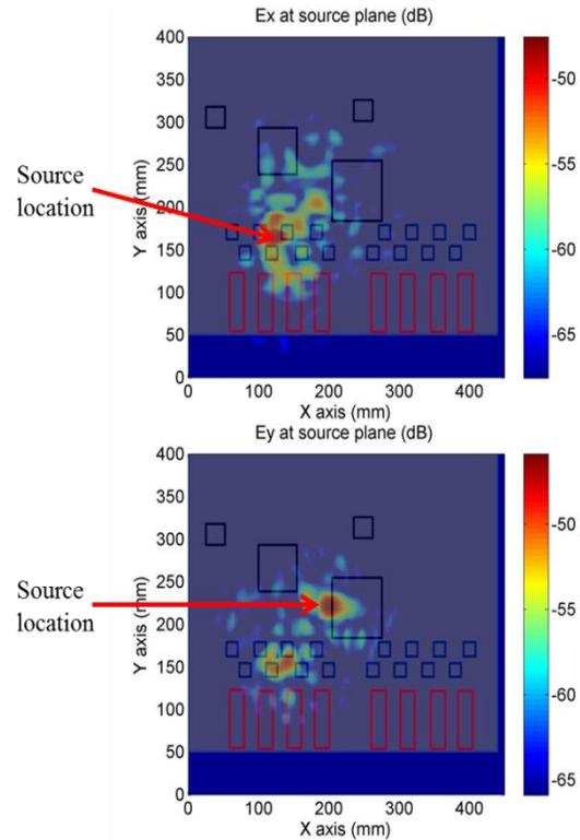
Fig. 6. Reconstructed  $E_x$  and  $E_y$  field component magnitude in dBm at the PCB plane.
