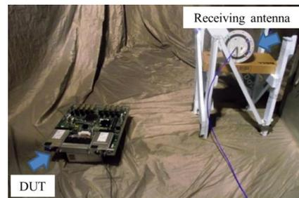
Fig. 9. Setup for the TRP measurement in a reverberation chamber
