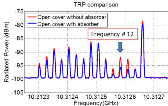
Fig. 9. TRP spectrums comparison with and without the absorber material.
