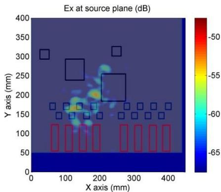
Fig. 8 a) Reconstructed  $E_x$  fields at the PCB plane, with absorber.
