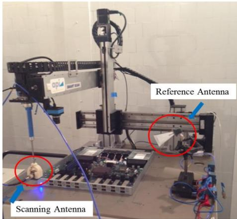
Fig. 2. ESM test setup for the real hardware measurement
