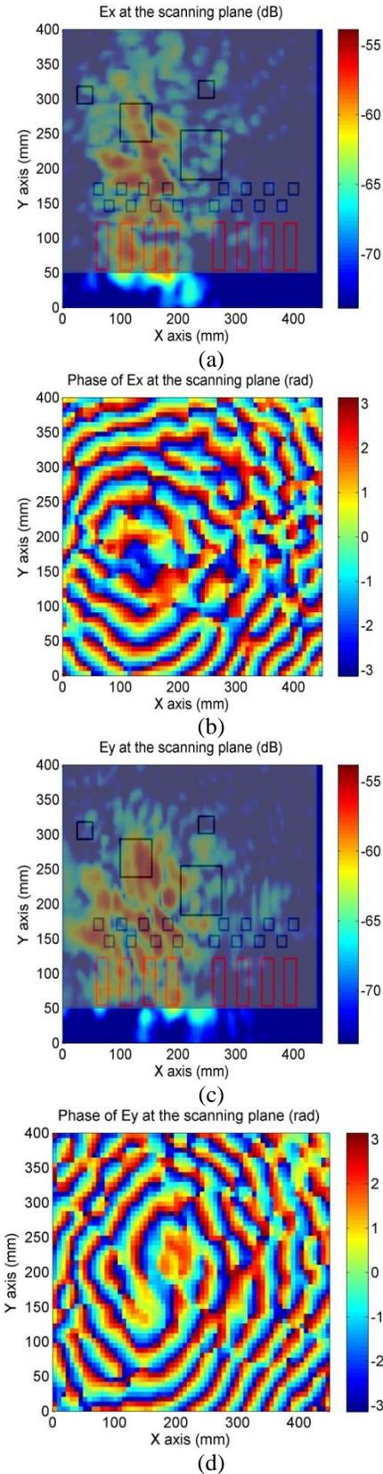
Fig. 4. (a) Measured  $E_x$  field magnitude in dBV (b) Measured  $E_x$  field phase in rad (c) Measured  $E_y$  field magnitude in dBV (d) Measured  $E_y$  field phase in rad at the scanning plane.
