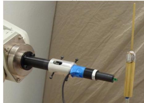
Fig. 17. Near-field scanning for a sleeve dipole antenna. (a) Measurement Setup. (b) photograph of probe and DUT.
