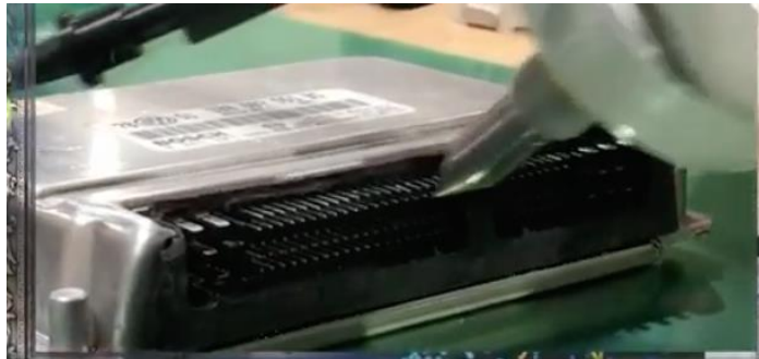
Automobile connector pin test by SmartScan-Pro
